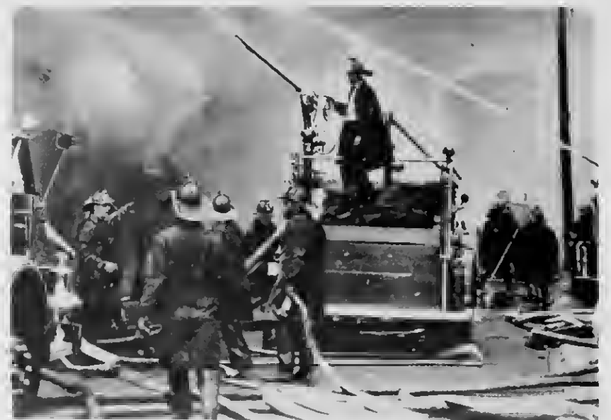
A FAR cry from the first pumping engine shown below is this modern piece of equipment that can pump 3000 gallons of water every minute and propel it hundreds of feet.
